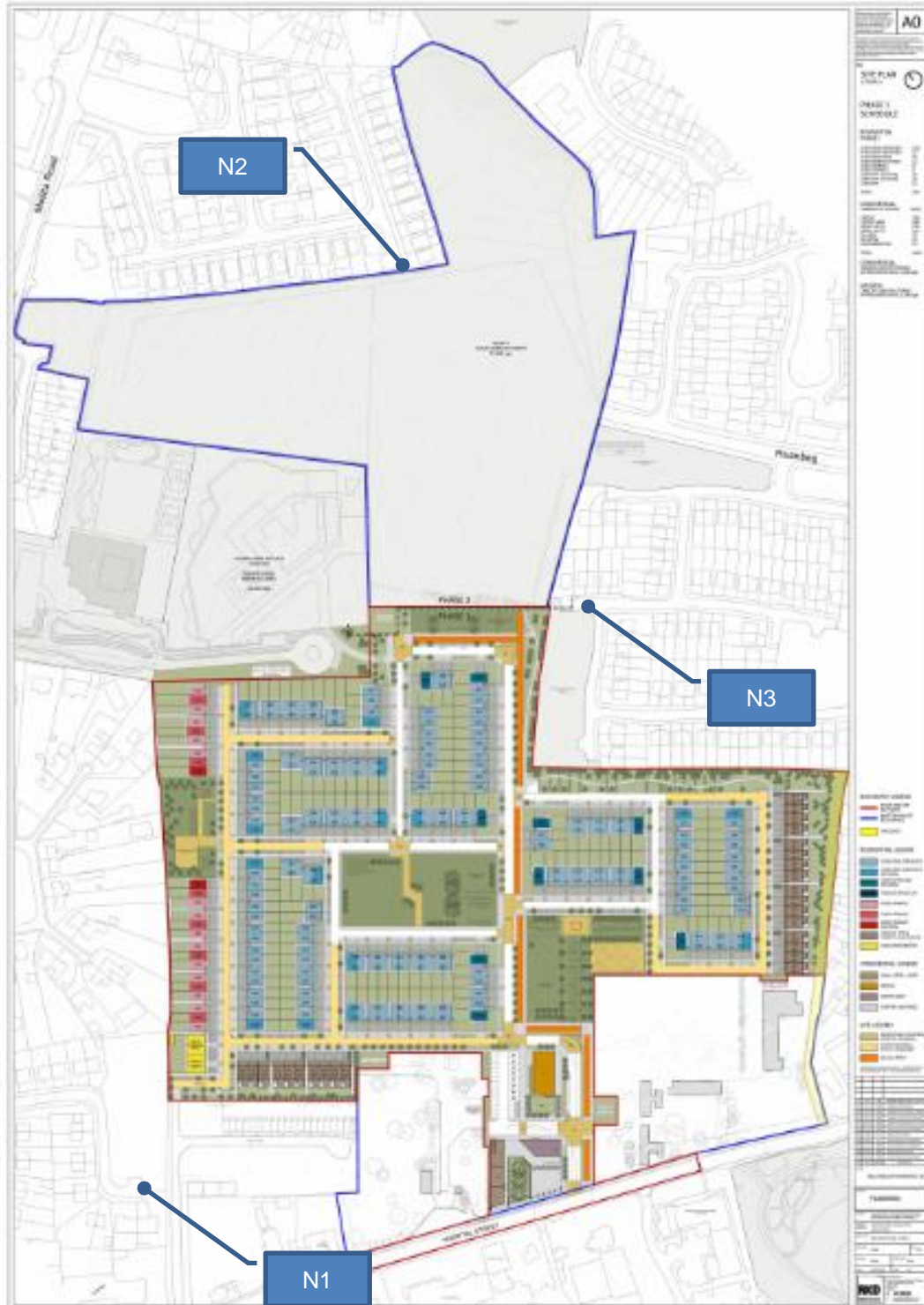
Fig. 11.1: Site context and noise monitoring locations
