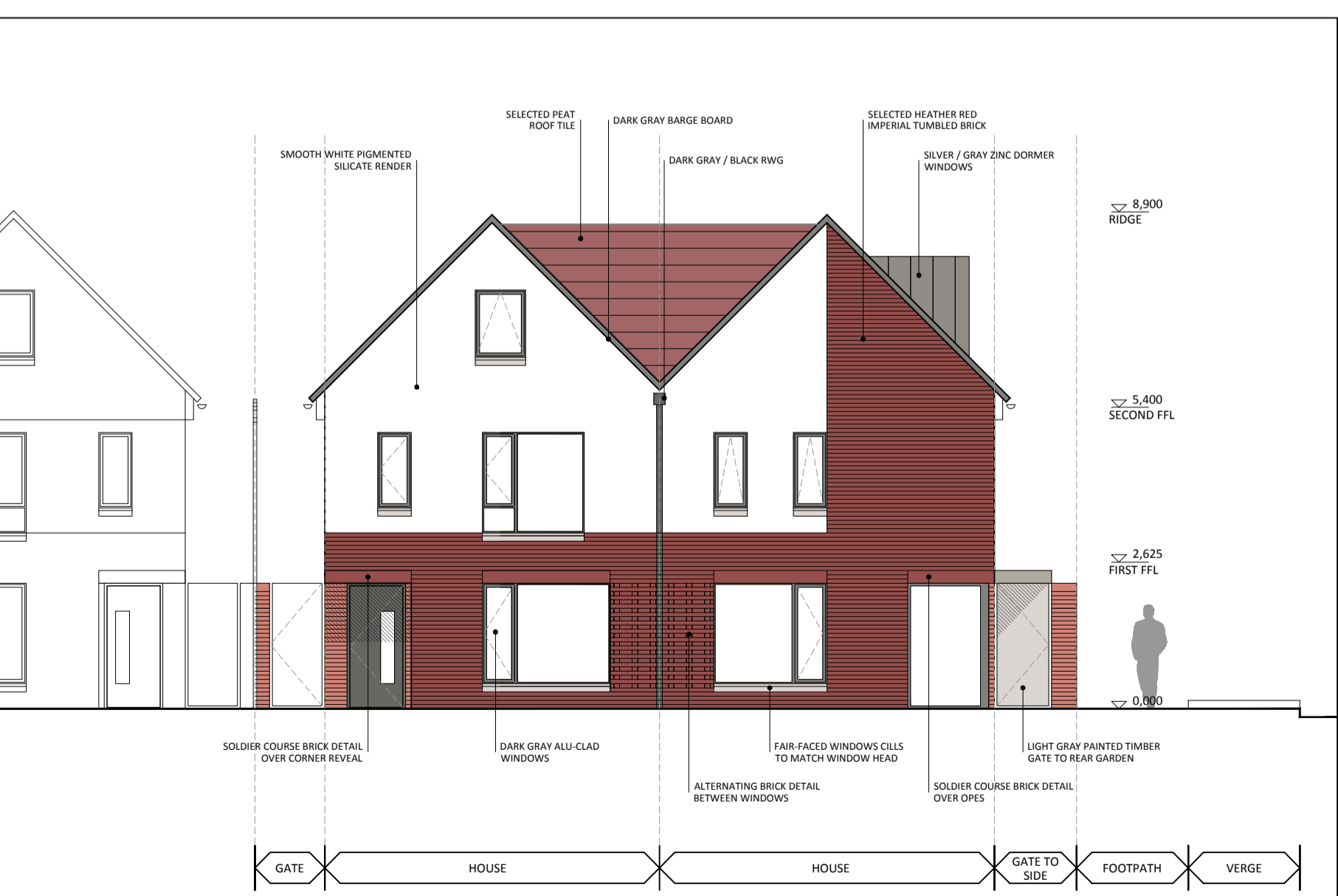
FRONT ELEVATION STREET / SIDE ELEVATION CORNER UNIT SELECTED (HEATHER) RED IMPERIAL TUMBLED BRICK
