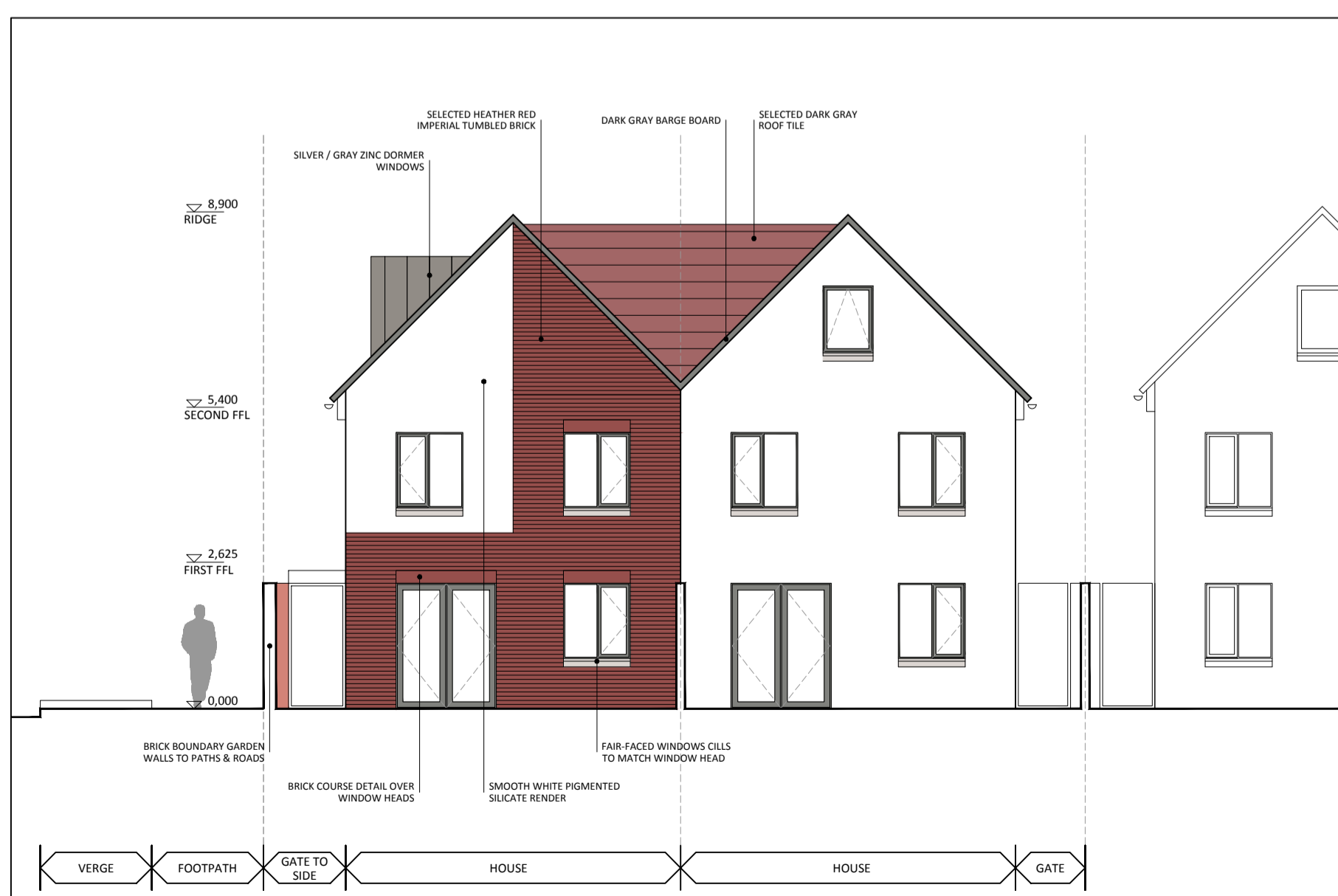
REAR ELEVATION SELECTED (HEATHER) RED IMPERIAL TUMBLED BRICK
